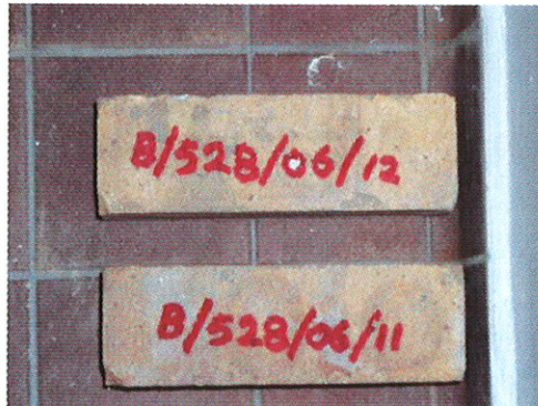
Photo A3-23 Shiral 60 AD - dark yellow fire bricks - Cremators Room and Storage Room
