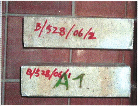
Photo A3-18 Shiral 60AD - Grey fire bricks, Cremators Room and Storage Room
