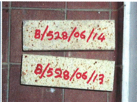
Photo A3-24 Shiral 60 AD - White dotted fire bricks - Cremators Room and Storage Room
