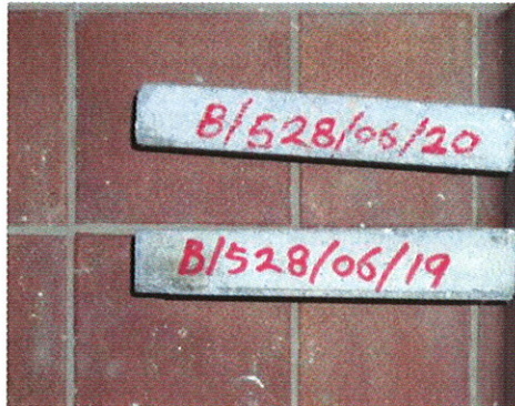
Photo A3-27 Shiraflo SC60 - Grey thin bricks - Cremators Room and Storage Room
